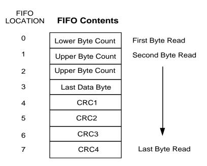
Figure 5.7.3 FIFO Alignment for 8 X N byte
