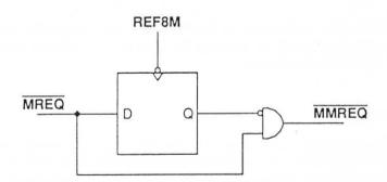
This logic modifies  $\overline{MREQ}$  from the ARM to produce  $\overline{MMREQ}$ , which is connected to the  $\overline{MREQ}$  input on MEMC. REF8M is a MEMC output. Without this change, MEMC may merge the first instruction prefetch following a multiply with the last cycle of a DMA or refresh operation, which will cause the instruction to be fetched from the incorrect address.
