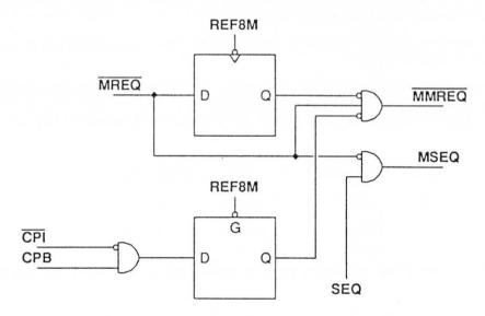
In addition, ARM or the Co-Processor must be allowed to drive the data bus for the register transfer cycle, and the system ROM must be prevented from driving the bus at the same time:
