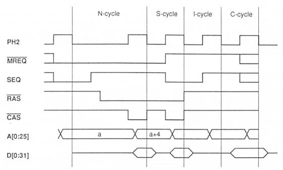
When an S-cycle follows an N-cycle, the address will always be one word greater than the address used in the N-cycle. This address (marked "a" in the above diagram) should be checked to ensure that it is not the last in the DRAM page before the memory system commits to the S-cycle. If it is at the page end, the S-cycle cannot be performed in page mode and the memory system will have to perform a full access. The processor clock must be stretched to match the full access.
