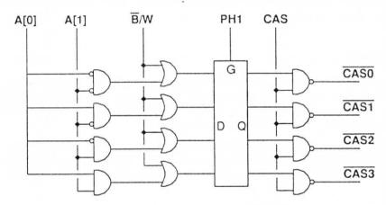
CASO drives the DRAM bank which is connected to D[0:7], CASI drives the bank connected to D[8:15], and so on. This has the added advantage of reducing the load on each column strobe driver, which improves the precision of this time critical signal.
