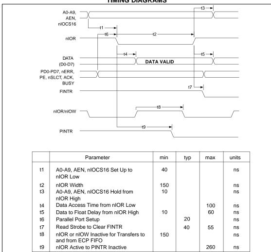
FIGURE 4 - MICROPROCESSOR READ TIMING
