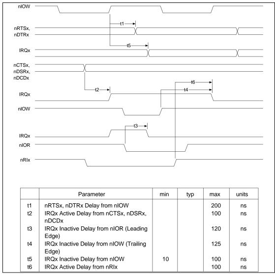
FIGURE 10 - SERIAL PORT TIMING
